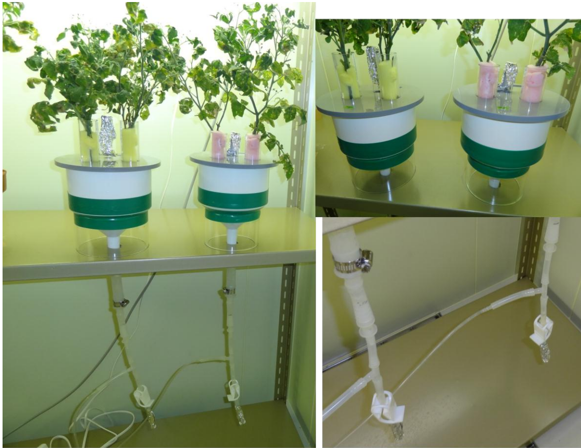
Fig. 3. The Hydroponic culture system
